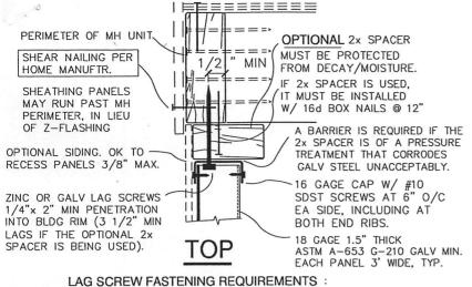
2 LAG SCREWS PER FOOT OF PANEL (EXCEPT AT VENTS), TYPICAL. LOCATIONS WITH DESIGN SNOW LOADS GREATER THAN 30 psf UP TO 120 psf REQUIRE 3 LAG SCREWS PER FOOT PF PANEL.
