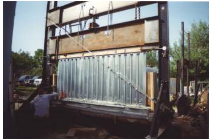
ICC-ER Combined-Loads Testing Setup
