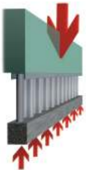
Load-spreading I-beam provides continuous support.
